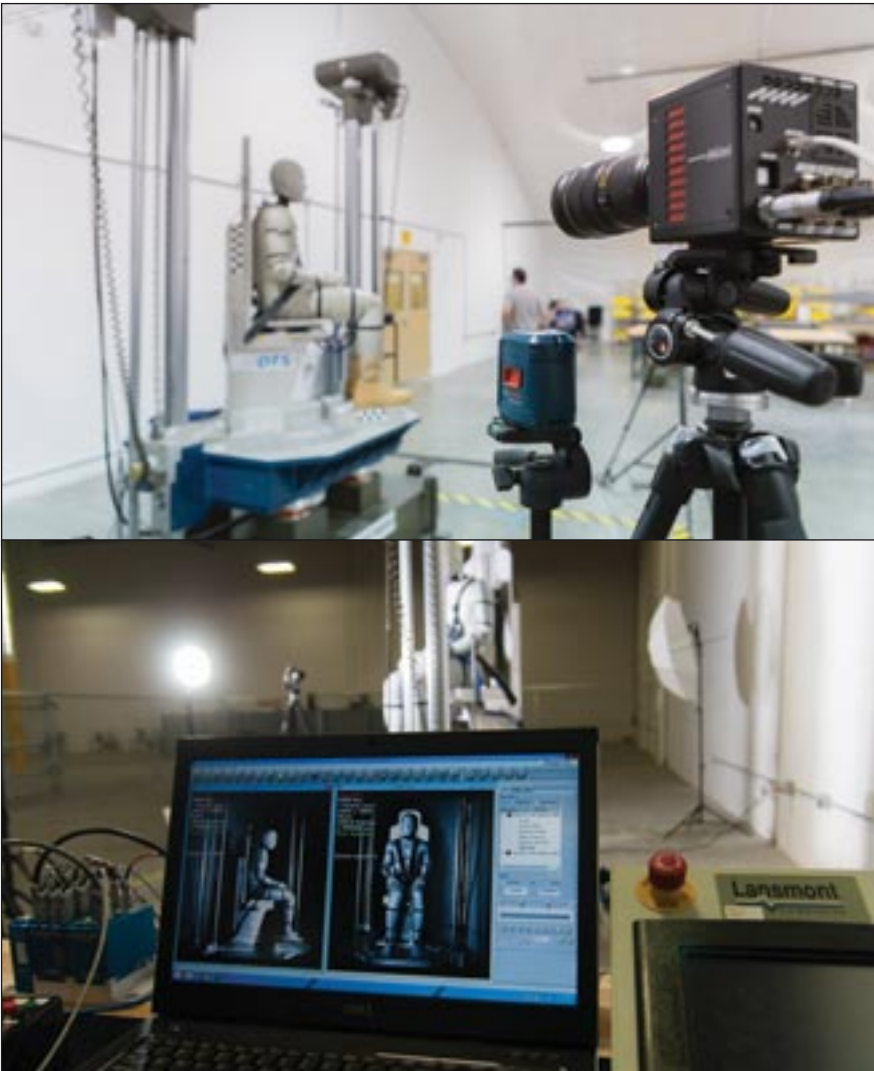
Multiple high speed cameras in the lab capture test images at 100,000 fps which allows the engineering team to track and map data with the movements on camera.
