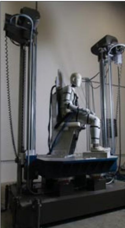
WIAMan, the first test dummy built specifically for under-body blast testing, is prepped on the drop tower for a validation test that will impart a 200 g pulse for 7 milliseconds, simulating an under vehicle blast.
